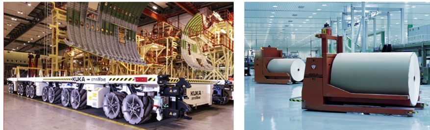
Fig. 7. Examples of laser guided vehicles (from left to right): KUKA industrial robots ( http://www.kuka-omnimove.com/ ), image obtained from [14], and Efacec AGV to transport paper reels at Soporcel ( http://www.efacec.pt/ ).
