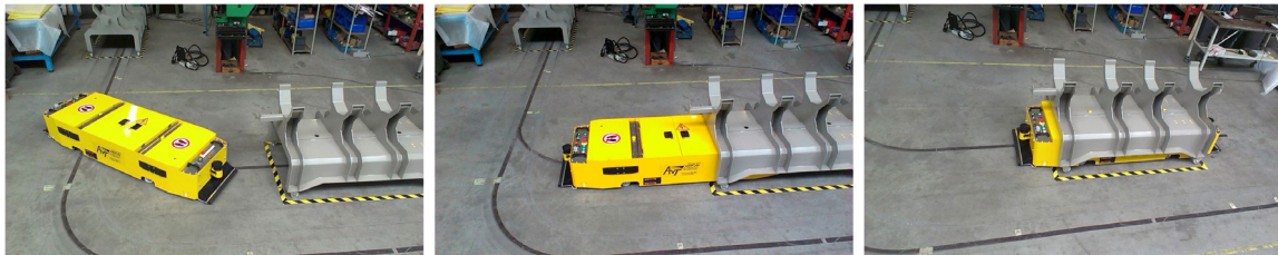
Fig. 5. Photos of an AGV designed and built by A-VT Europe NV using line guidance ( http://www.a-vt.be/ ).
