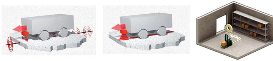
Fig. 2. Line guidance principles (from left to right): wire and optical guidance ( http://www.goetting-agv.com/ ) and magnetic tape guidance ( http://www.transbotics.com/ ).
